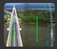
Valid speed detection at 600 m / 1968 ft, ANPR/LPR up to 150 m / 490 ft (nighttime up to 100 m / 328 ft).
